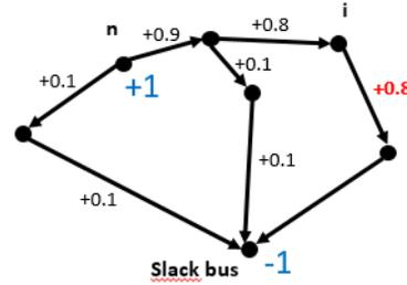
Fig. 1. Example of PTDF on a small network
